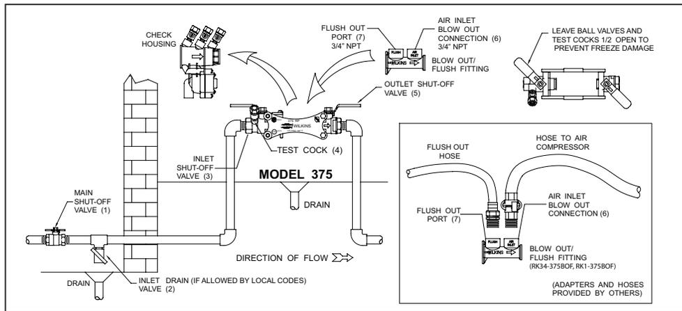
**To Blow Out System for freeze protection, use the following procedure:**
